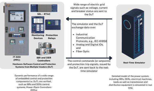
Embedded control and protection systems are the combination of hardware and software platforms, e.g., Power-Plant-Controller (PPC), IBR and DER controllers, and protection relays
